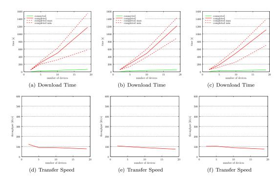
Figure A.4: Measurement 4: Single file approach, one-time synchronization, discovery interval 2 sec
