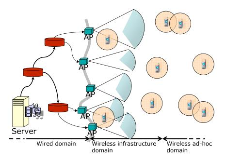
Figure 1.1: Contents are provided by means of podcast via access points and they are redistributed in the ad hoc domain.
