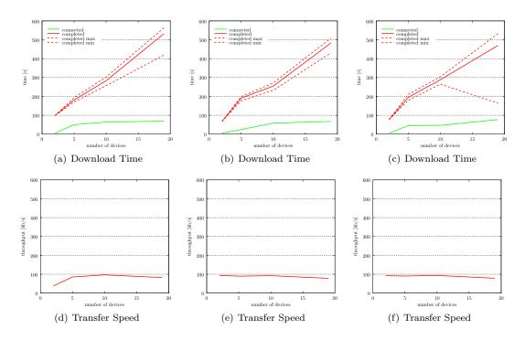
Figure A.3: Measurement 3: 100 small files, synchronization every 30 seconds, discovery interval 2 sec
