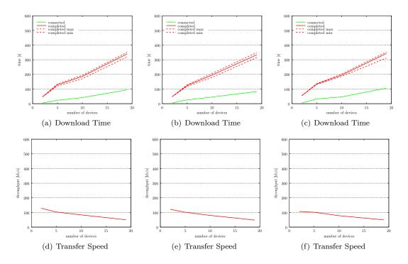
Figure A.7: Measurement 7: Single file, intelligent synchronization, discovery interval 2 sec
