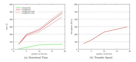
Figure 6.12: 100 small files: synchronization every 30 seconds, discovery interval 2 sec
