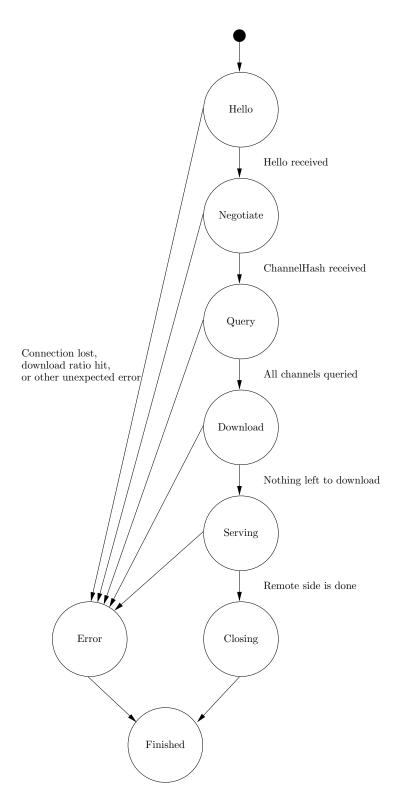
Figure 3.2: TransferServer / TransferClient state diagram
