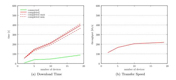
Figure 6.8: Single file distribution: synchronization every 30 seconds, discovery interval 2 sec
