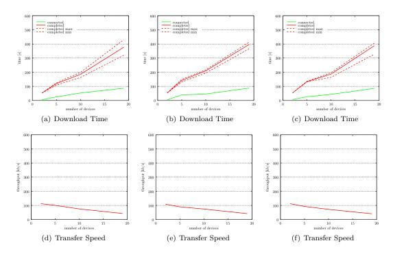
Figure A.2: Measurement 2: Single file, synchronization every 30 seconds, discovery interval 2 sec
