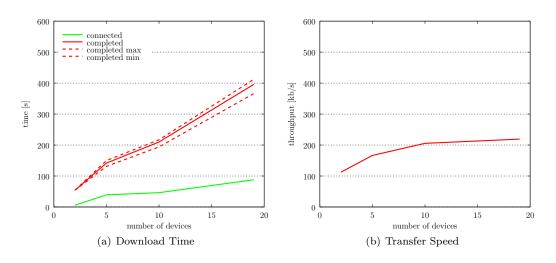
Figure 6.13: Single file: synchronization every 30 seconds, discovery interval 2 sec, ratio 1MB/synchronization
