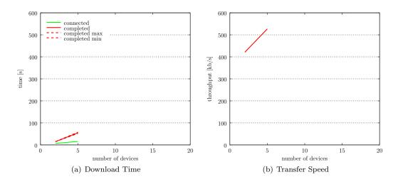
Figure 6.10: Single file with laptops: synchronization every 30 seconds, discovery interval 2 sec
