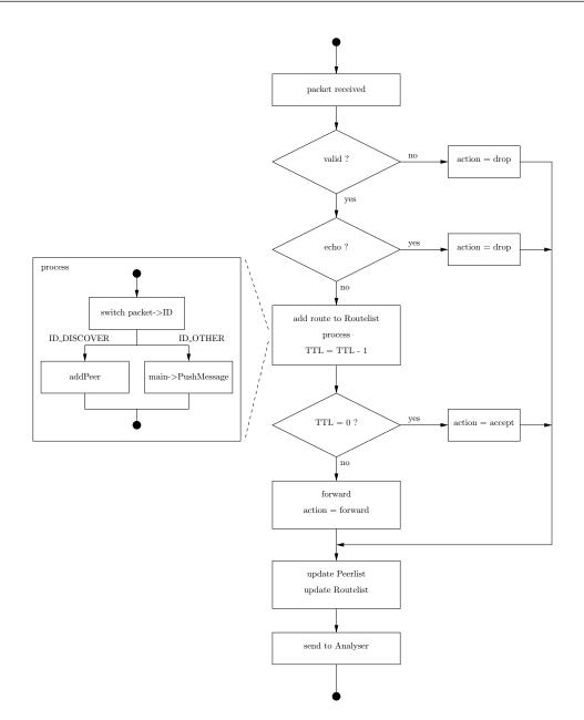
Figure 4.1: Router::Update() flowchart for UDP packets received from the network
